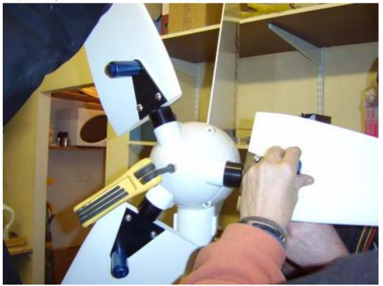
The holes in the blades are a deliberately tight fit and it may be necessary to turn the fasteners as they are inserted, or even to ream through with a hand drill. First loosely fit all the nylock nuts by hand, then fully tighten with a spanner. The torque on a M8 is 21.5 Nm. Finally, recheck the tightness of all the nuts.
