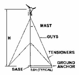
**Tensioners:** These are the simple and easiest method of tensioning guys, but adjustment must be uniform, since it is the guys that resist the thrust of the wind turbine. Do not over tension – a guy should be snugly taut, but not drum tight.
