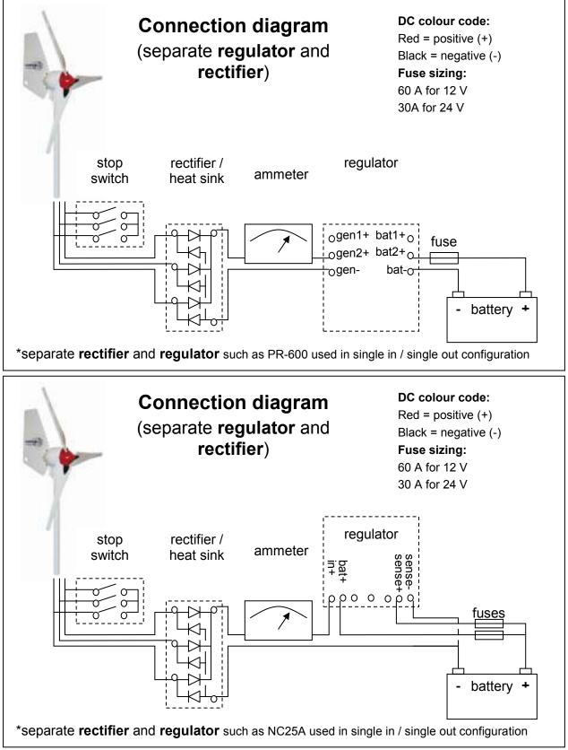
If the Ampair 600 wind turbine is connected on the load side of the battery isolator switch, it may damage electrical equipment. Under these conditions it is possible to run the wind turbine whilst the battery is isolated, but this can subject the system to excess voltage.
