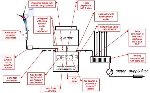
electrical grid as well as to battery systems. In this mode the turbine is connected to a G83/1 grid tie inverter via an interconnection unit which houses the rectifier, stop switch, metering, etc. The interconnect unit eases the task of the installing technician. These grid-connected units are only suitable for use with interconnect units and inverters supplied by Ampair, and installed by personnel trained by Ampair.
