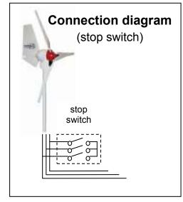
We recommend installing a 'stop' switch which should be more correctly thought of as a 'parking' switch. Just as the parking brake in a car should not be relied on to stop a car at high speed, so the parking switch of the Ampair wind turbine should not be relied on to stop the rotor disc in high winds. Instead it is best to apply it before the arrival of very high winds, or if needing to ensure that the rotor does not move in low winds (e.g. when approaching the rotor for maintenance).
